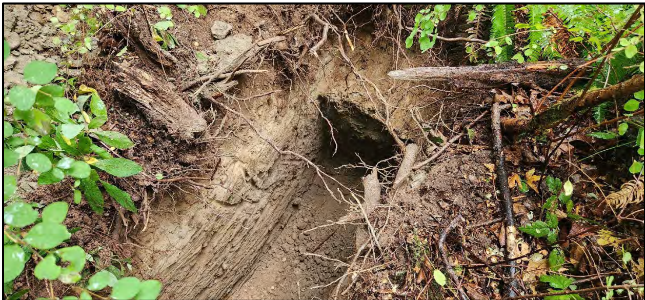
Image 2: Subsurface conditions as observed in TP-2. Note dense, undifferentiated glacial deposits materials extending to depth from near surface elevations. Photo taken July 29 th , 2024
